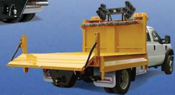
If your application requires easy side and rear access, the MSO-2 & the MSOE-2 are for you. The two drop sides combined with the double-acting door, greatly increase their versatility. The grade 50 steel used in their respective construction, provides both models necessary ruggedness to do the job while maintaining weight to a minimum.
